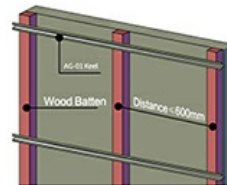
2. FIX AG-01 KEEL ON WOODEN BATTENS
