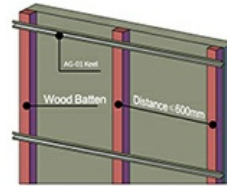
2. FIX AG-01 KEEL ON WOODEN BATTENS
