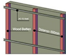
2. FIX AG-01 KEEL ON WOODEN BATTENS
