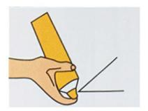
4.Invert the sprinkler irrigation after use andspray downward forabout 2-3seconds to clean the residual glue and avoid clogging of the spray head
